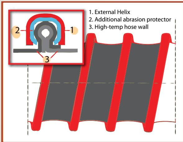
The Crushproof® CF is a super lightweight, flexible exhaust hose with 1:5 compressibility and a small bend radius. It is resistant to mechanical load, abrasion, and vibration. It can handle exhaust temps up to +570°F when used with proper adapters, so it works well with diesel engines. It is a great choice for reels as well. The chart below shows our size options and basic specifications. **HOSE MUST BE USED WITH A FAN.**
