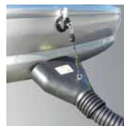
Adapters are critical to proper exhaust system function and for prolonging hose life. A hook and chain holds the adapter in place during use. At least 1/2" diameter difference between pipe and adapter is required for proper performance. Please refer to the information below for proper sizing.
